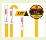
Line markers like these display the name of the pipeline operator and the telephone number where the operator can be reached in the event of an emergency. Even if you don't see one of these markers. there may still be natural gas lines nearby. Always call 811 before you dig! Not all line markers are represented in this illustration.
